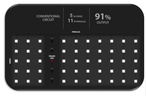
LUX GUARD by TRT is a **patented** current sharing PCB and circuit design philosophy. If an LED fails then its current is shared via neighbouring circuits, with each LED's brightness increasing slightly to compensate. LUX GUARD ensures that a luminaire continues to provide its designed lumen performance, even in the case of nuisance LED failures, and reduces the maintenance costs of a project.
